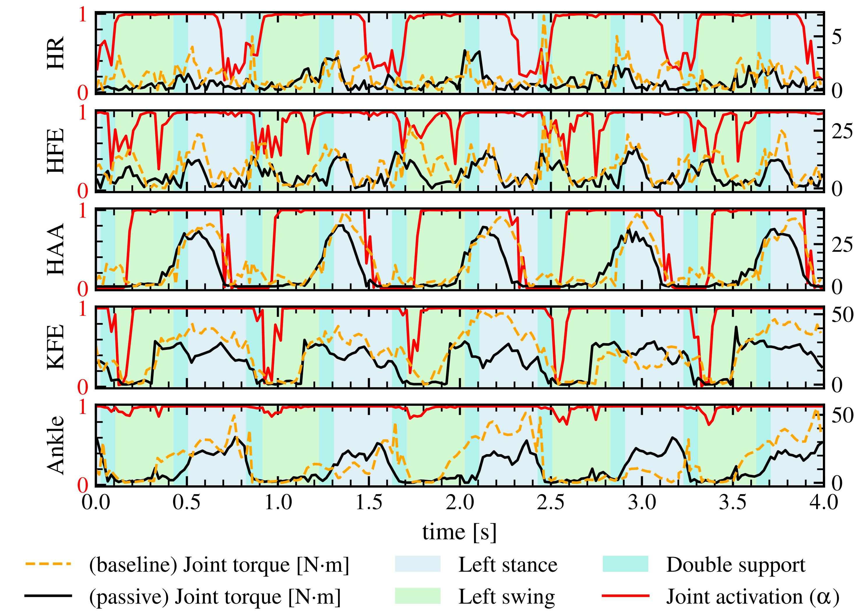
**Comparison of left leg absolute joint torque for real-world baseline vs. passive walking:** KFE deactivation during swing in passive walking demonstrates the utilization of passive dynamics, contrasting with the generally higher torque of the baseline policy
