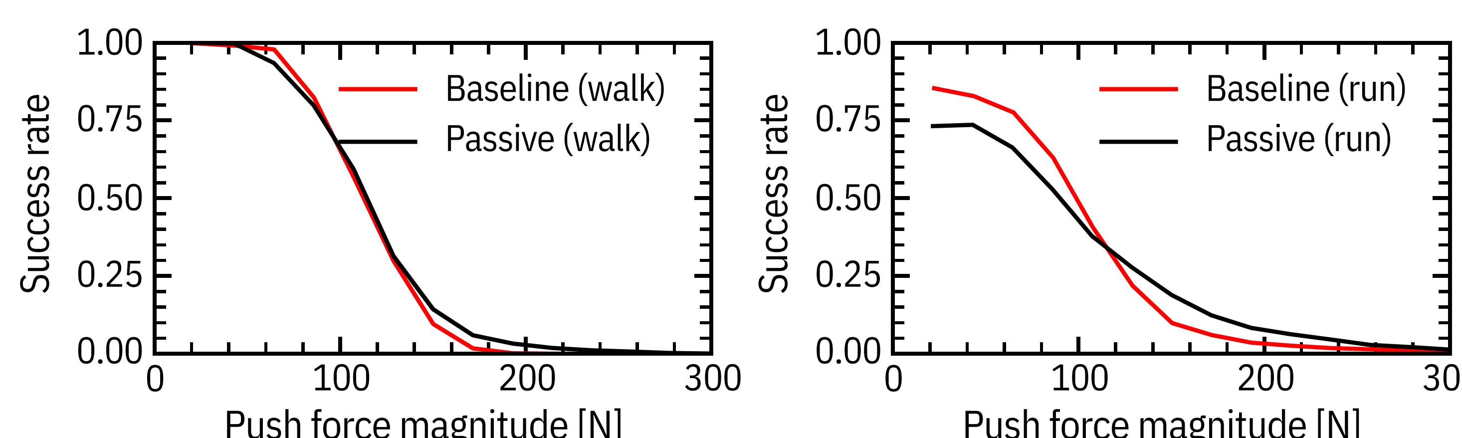
**Push recovery in simulation:** baseline vs. passive policy for walking (left) and running (right). Adding passive actions leaves robustness largely unchanged.
