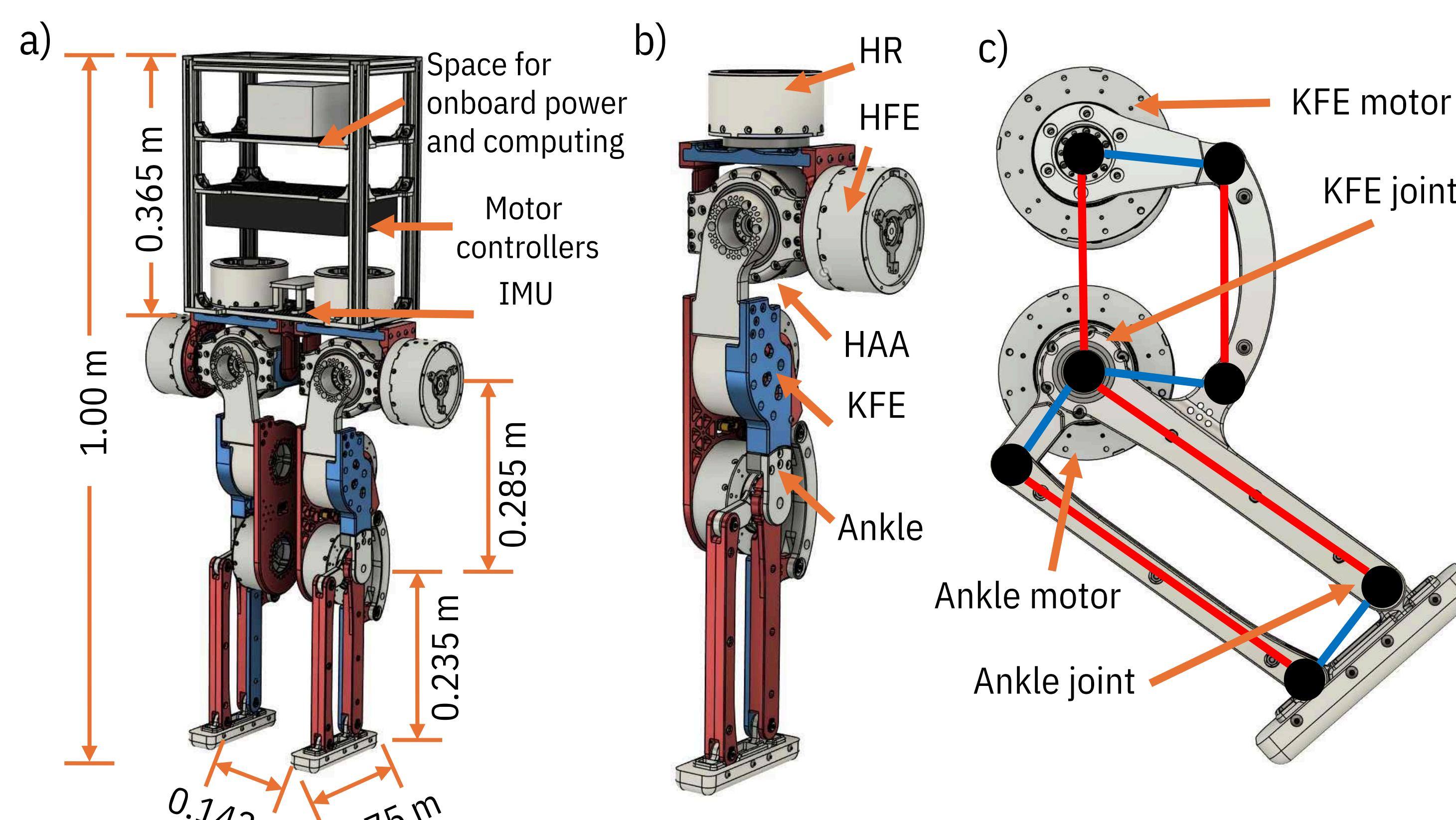
**Mechanical Design Overview:** a) Major dimensions and the extensible body design. b) All joints in the left leg. c) Two parallel linkages in the knee and ankle.
