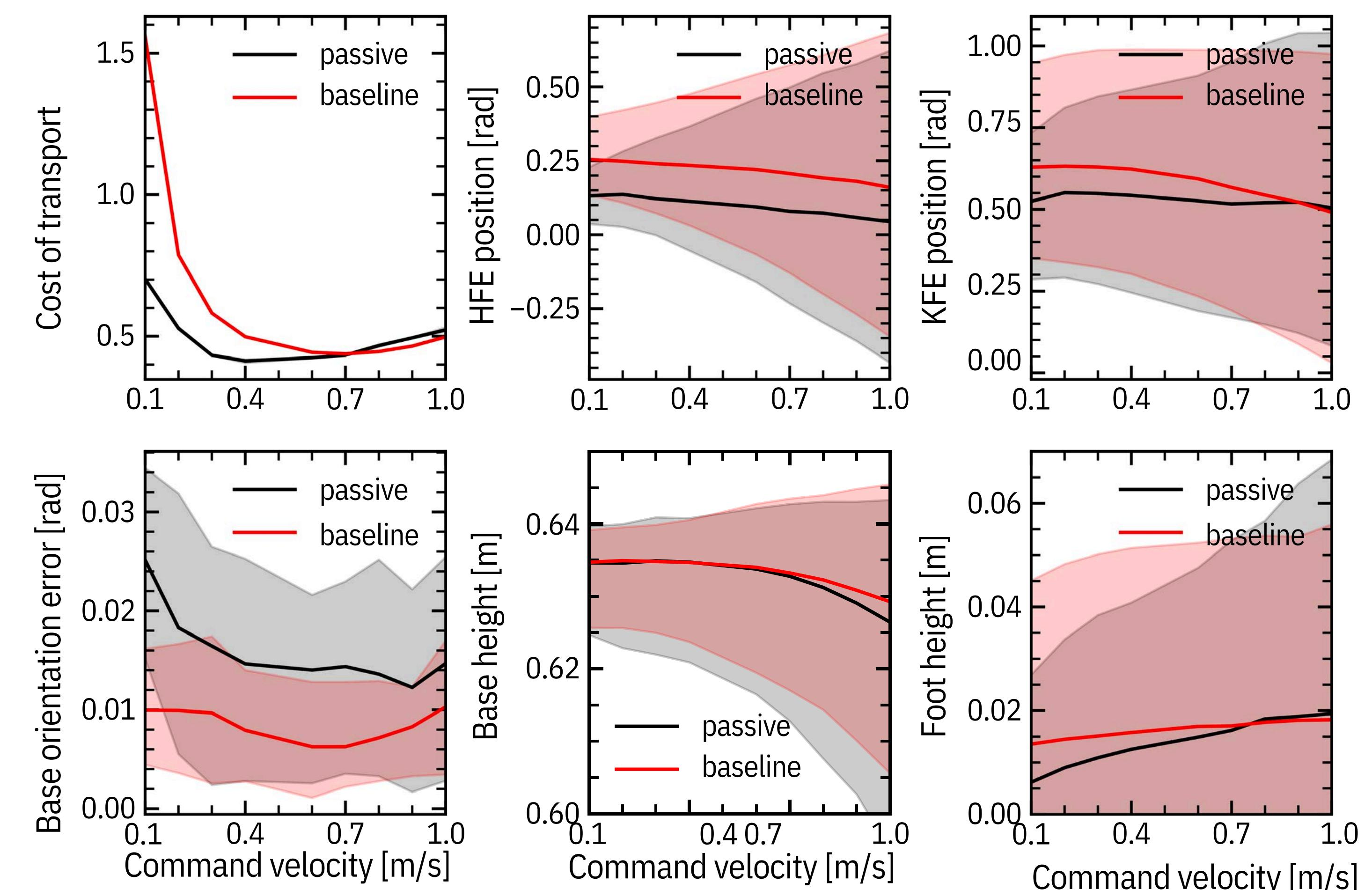
**Baseline vs. passive walking policy in Simulation:** Passive is up to 50% more energy-efficient at low speed, with reduced KFE/HFE positions (less action). Shaded regions show 95% confidence intervals.
