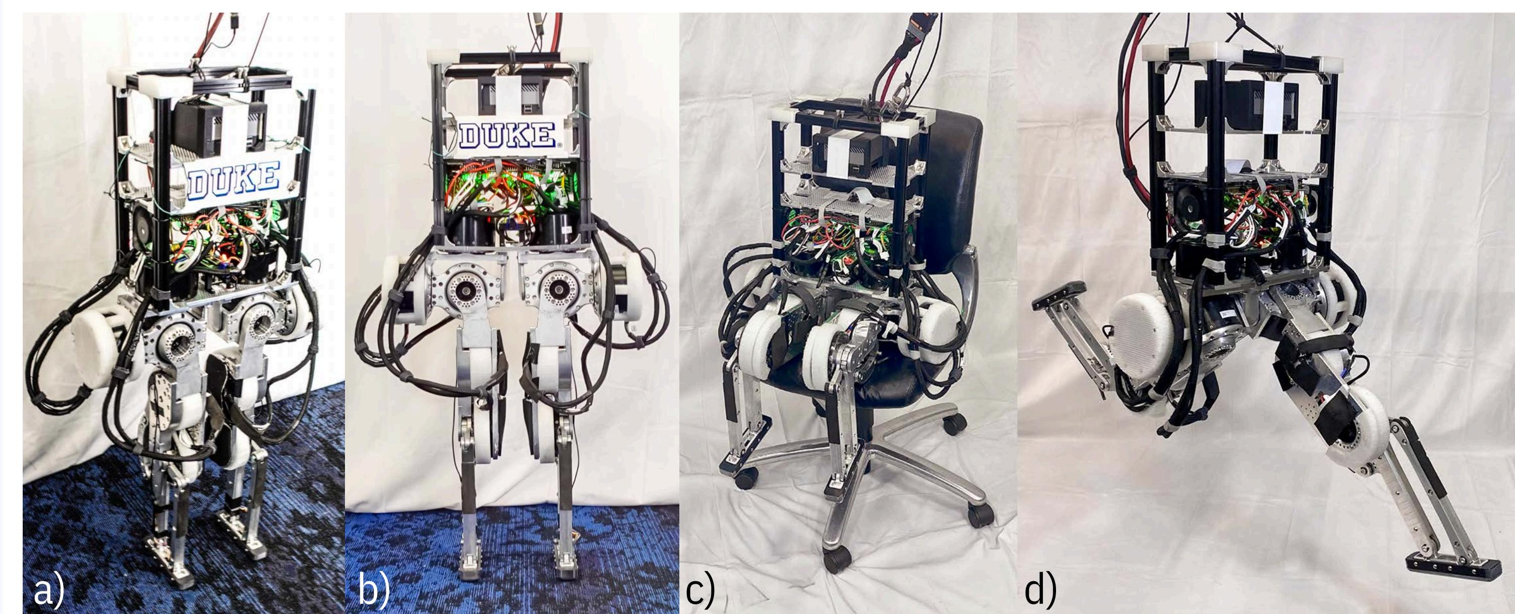
**Duke Humanoid V1:** a) and b) The frontal plane symmetry of the hip enables static standing with straight knees. b) and c) Additional poses demonstrating the robot's range of motion.
